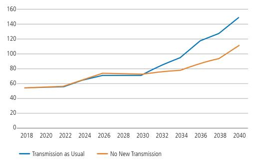
Under a low-carbon future scenario, results from ReEDS show that transmission with Canada becomes increasingly important for sustaining emissions reductions and has a significant impact on the generation mix in border regions. In ISO New England, greater cross-border transmission capacity reduces domestic natural gas generation. In New York ISO, additional transmission capacity with Canada is associated with an increase in domestic renewable generation.
